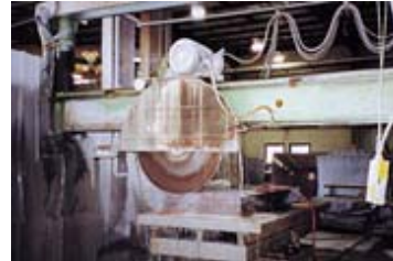
Equipment at the North Kingstown plant includes bridge saws from Loeffler and other German manufacturers.
